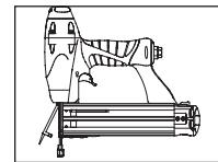
7. Push button down again to lift the hook. Close the door and release the button to reengage the hook with the nose.
