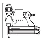
6. Remove the tool from the work surface. The Work Contact Element (WCE) must return to its original down position. The tool **MUST NOT OPERATE**. Do not use the tool if it operates while lifted from the work surface. Personal injury may result.
