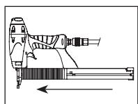
5. Always unload all fasteners before removing tool from service. Unloading is the reverse of loading, except that you must **disconnect** the air supply before unloading.
