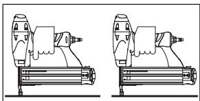
against the work surface. Pull the trigger. The tool **MUST OPERATE.**
