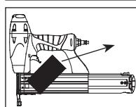
3. Make sure the trigger and work contact element (WCE) move freely up and down without sticking or binding.
