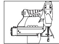
8. Make sure the trigger and work contact element (WCE) move freely up and down without sticking or binding.
