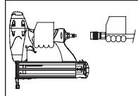
5. Depress the Work Contact Element (WCE) against the work surface without pulling the trigger. The tool **MUST NOT OPERATE**. Do not use the tool if it operates without pulling the trigger. Personal injury may result.
