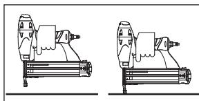
a fastener is driven. The tool can be actuated by depressing the WCE against the work surface followed by pulling the trigger.
