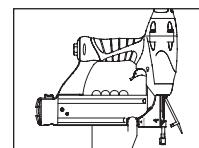
4. The door can now be rotated, exposing the jammed fastener.
