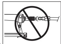
*air in the tool is discharged at the time the fitting or hose coupling is disconnected. Do not use a check valve or any other fitting which allows air to remain in the tool. Death or serious personal injury could occur.*
