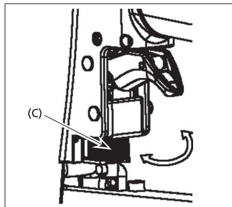
3. For deeper penetration, turn the wheel (C) to left to the extent desired.
